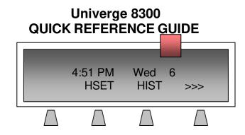
**HSET** If you are using a headset, press the **HSET** soft key to receive dial tone or answer a ringing call. Press **HSET** again to hang up. Otherwise, you may lift the handset or press the **Speaker** button. To talk hands-free, make sure MIC button is lit red. You may press the **MIC** button or the **MUTE** soft key to mute or un-mute during the call.
