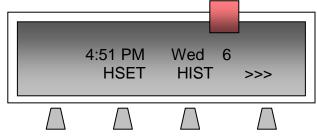
**HSET** If you are using a headset, press the **HSET** soft key to receive dial tone or answer a ringing call. Press **HSET** again to hang up. Otherwise, you may lift the handset or press the **Speaker** button. To talk hands-free, make sure MIC button is lit red. You may press the **MIC** button or the **MUTE** soft key to mute or un-mute during the call.
